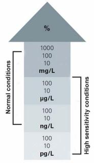
Figure 2: Normal conditions: Best suited to heavy matrices ideal for trace level determination. High sensitivity conditions: Ideal for ultra-trace level determination well suited to semi-conductor applications.
